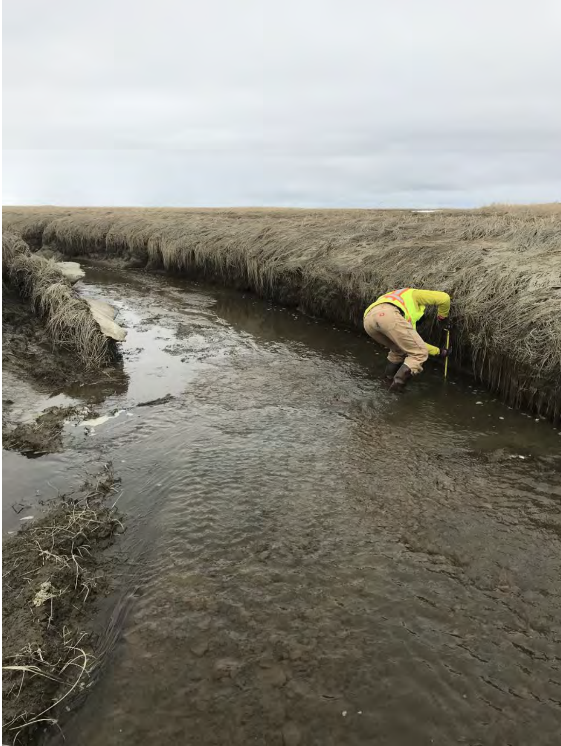
Figure 4. Creek downstream of runway culvert outlet. Nearly vertical banks indicate tidal influence.
