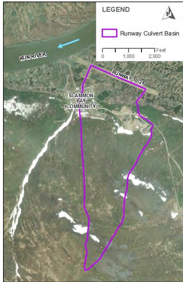
Figure 3: Runway Culvert Basin
